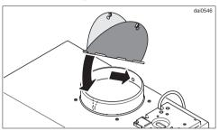
If the on-site ventilation system does not have a **non-return flap**, then the non-return flap supplied with the appliance must be fitted in the exhaust socket in the motor unit.
